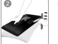
Hold the main body of the product with your hand as shown by the figure. Pull the stand in the direction of the arrow as shown in the figure to separate it.
